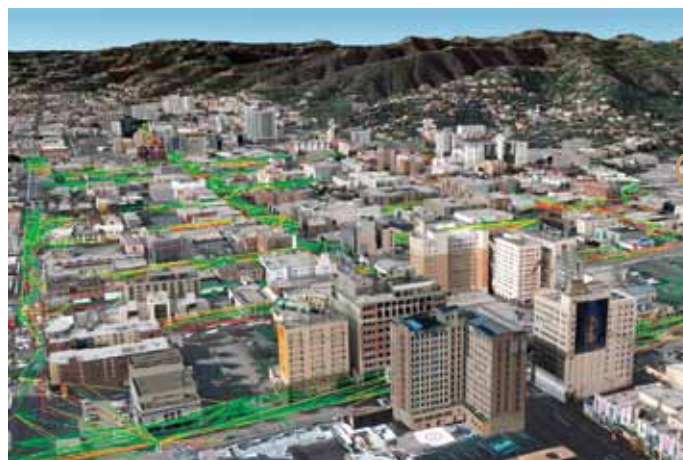
SMART STREETS: The city of Hollywood is using sensor technology to ease the pain of urban parking. Wireless mesh networks, embedded in the city’s streets, alert drivers to available parking spots via their mobile devices. The city can also use the networks’ data to determine which cars have exceeded their metered parking times. The colored lines shown here represent throughput, signal strength and other parameters.
