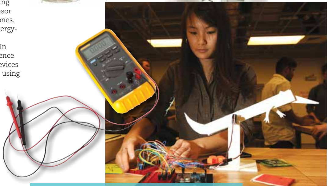
Third-year EECS major Brittany Cheng makes some adjustments to Tea-Rex, a device programmed to steep the perfect cup of tea. Motors connected to an Arduino controller raise and lower the neck of the apparatus while making use of time and temperature sensors.
